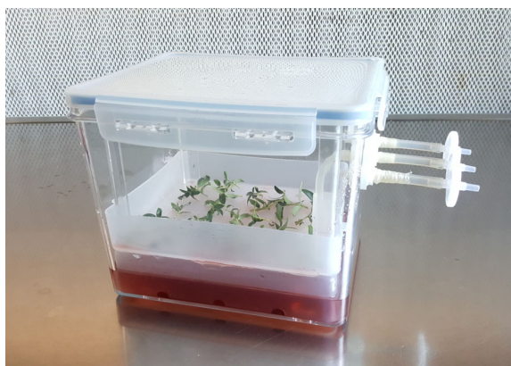
FIGURE 3 Temporary Immersion System by Plantform ™ bioreactor for olive shoots proliferation.
